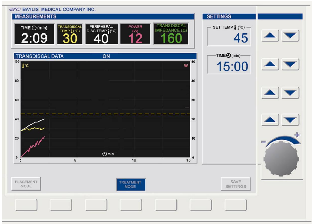
Figure 12: Generator graph of a poor procedure.
