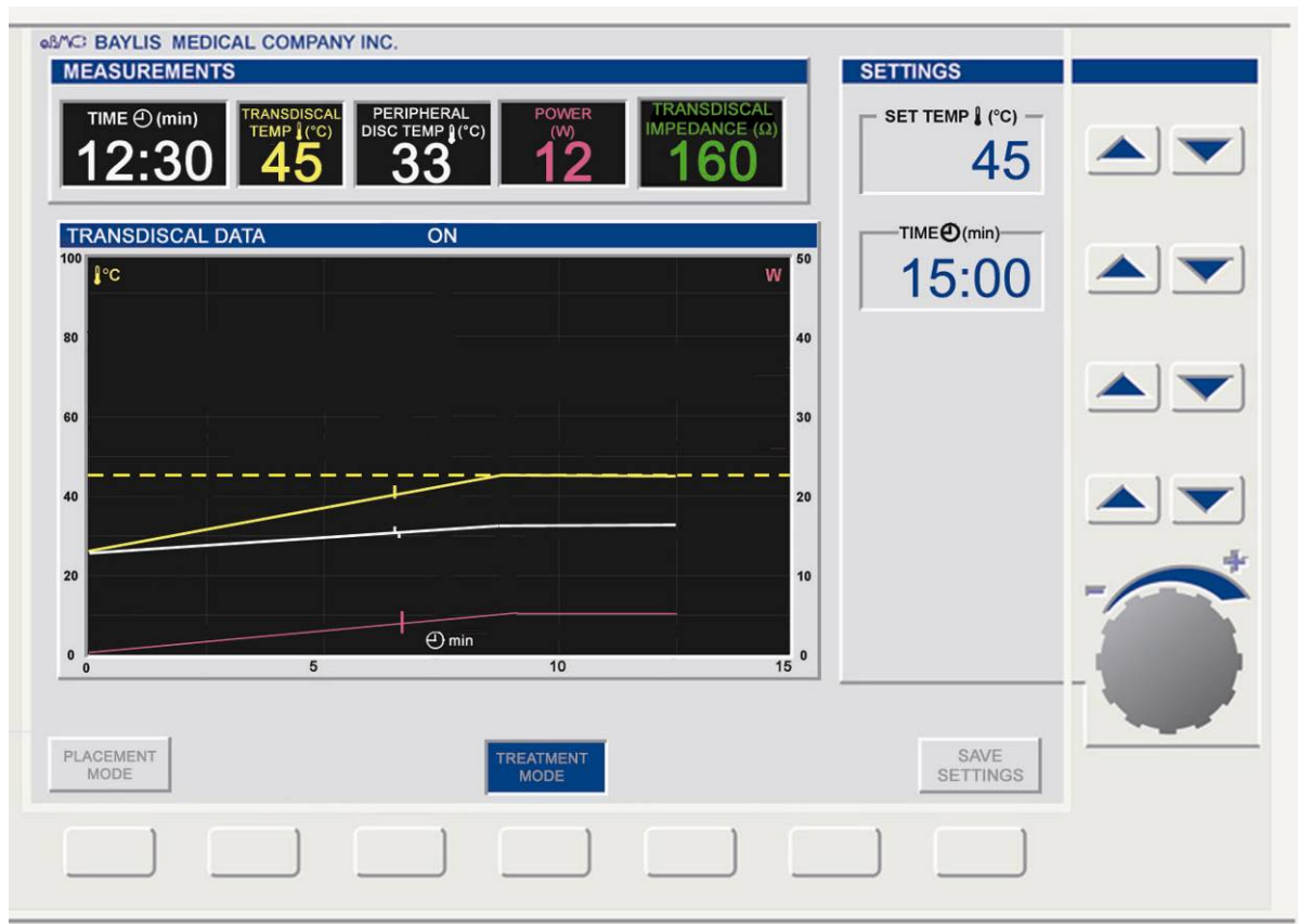
Figure 11: Generator graph showing a small blip is okay.
