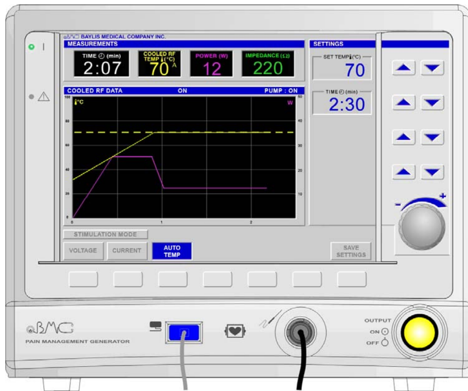
Generator graph showing that reaching the power limit is okay.
